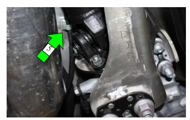
6. Remove the rear calipers by unbolting them (6). As with the fronts, don't disconnect the hose yet, but do set the caliper in a way that won't put any stress on the hose.
