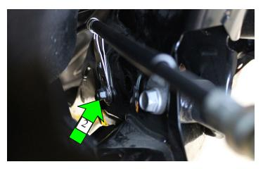
3. Driver's side: Pop the plastic retainer out of the heatshield (3). On the underside of the plastic piece, pull the two sides apart, then spin them around the housing in opposite directions to remove it from the housing. Kits without parking brakes should remove the cables altogether.
