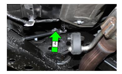
**5. Passenger's side:** Like on the driver's side, pop the plastic retainer out of the heatshield (5) and remove it from the cable. Kits without parking brakes should remove the cables altogether.
