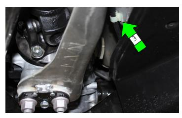
4. Passenger's side: Remove the bracket (4) that holds the cable to the subframe - just chase the parking brake into the car to find the bracket. This bracket is similiar to the one removed from the driver's side. Remove the plastic sleeve as well.
