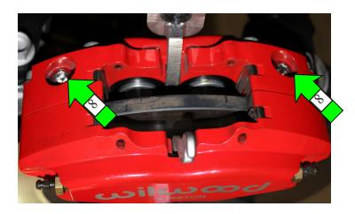
11. Smear a little thread sealant on the fitting that threads into the caliper (don't get any on the first two threads). Thread the fitting into the caliper until it's finger tight, then go 1.5 - 3 turns farther. These are tapered threads, so don't expect it to visibly bottom out on anything (the fitting in the picture is tight). Don't overtorque! (The brake line shouldn't be installed yet.)
