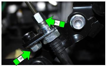
9. Slip the new hose into the bracket and line it up with the fitting. Get the stock fitting finger-tight (or something close), then reinstall the bolt (8). Tighten the stock fitting to 10 - 16 ft-lb.
