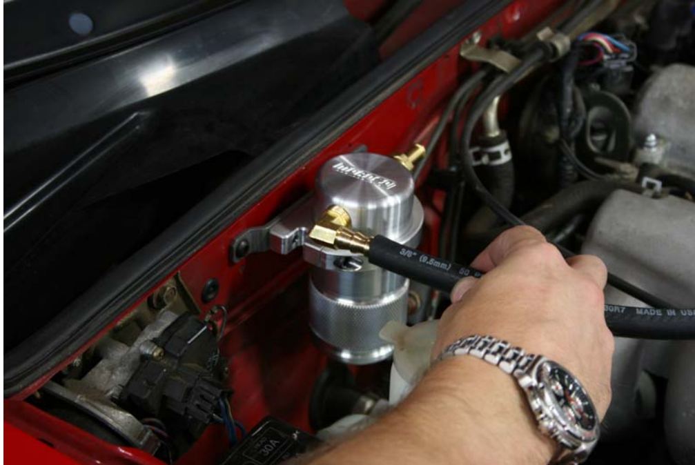
Step 17: Install other end of hose to Air Oil Separator as shown
