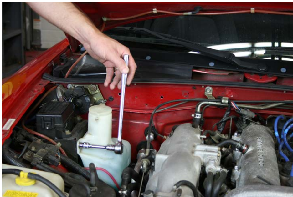
Step 9: Reinstall windshield washer tank mounting bolts
