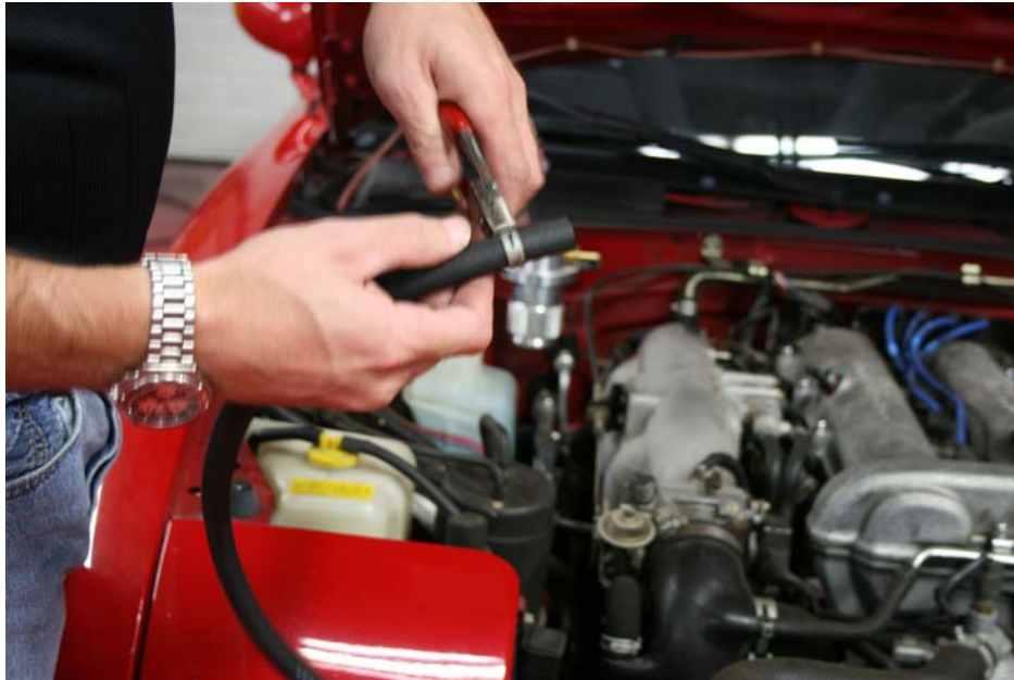
Step 15: Install (1) hose clamp on one end of 19" hose
