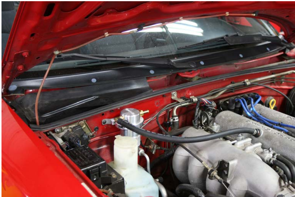
Step 17: Install other end of hose to Air Oil Separator as shown
