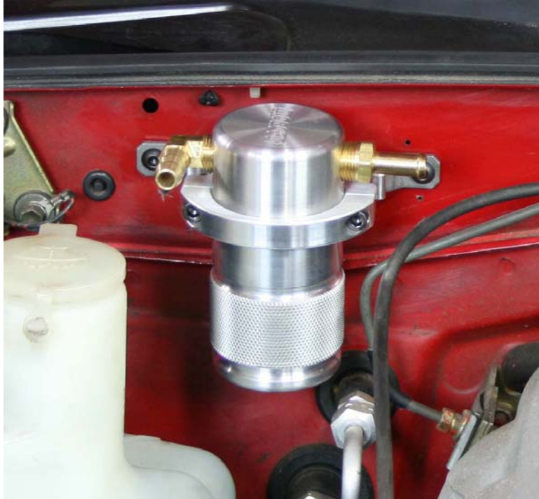
Step 10: Install Air Oil Separator using (2) \frac{1}{4} x 20 x \frac{5}{8} x BHCS
