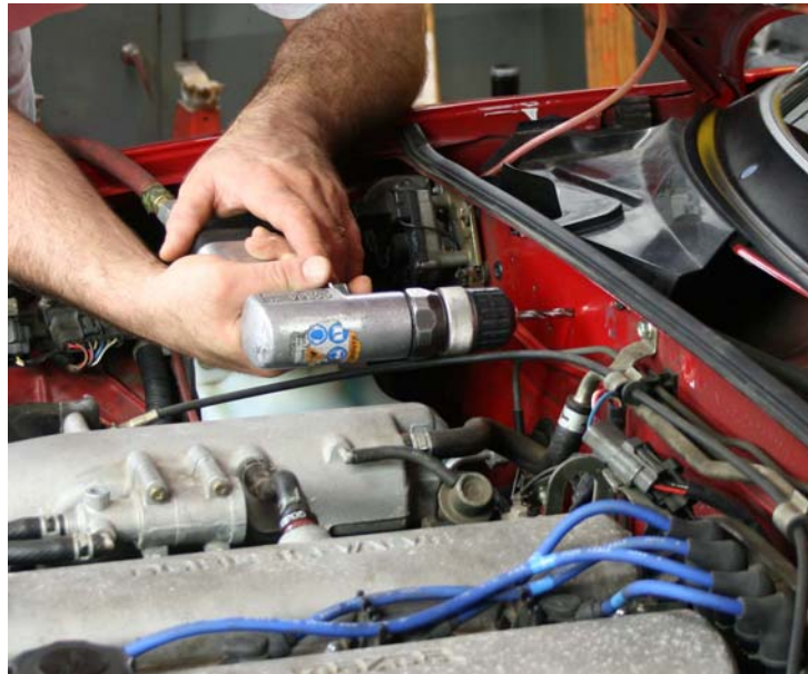
Step 7: Drill first 1/4" hole at marked location
